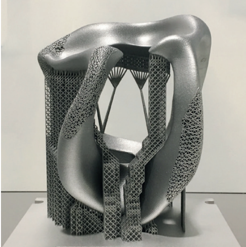
Fig 1: AlSi10Mg demo part manufactured in segments with dynamic adaptive parameter sets (AMCM M 290-2 1kW). Volume rate: 24 up to 64 mm 3 /s Source: EOS Innovation Center Düsseldorf
