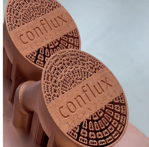
Fig 2: CuCP demo part (AMCM M 290-2 1kW). Source: Conflux technology
